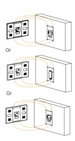
Tilt the device 15° and align the grooves on the back cover with the hooks on the bracket.
