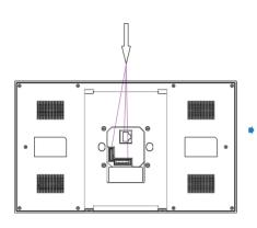
Plug the cables from the wall into corresponding interface on the back cover to test the device whether works properly.
