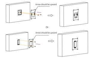
Fix the wall-mounting bracket on the 86 embedded box with two M4x30 crosshead screws, please ensure the bracket against to wall.
