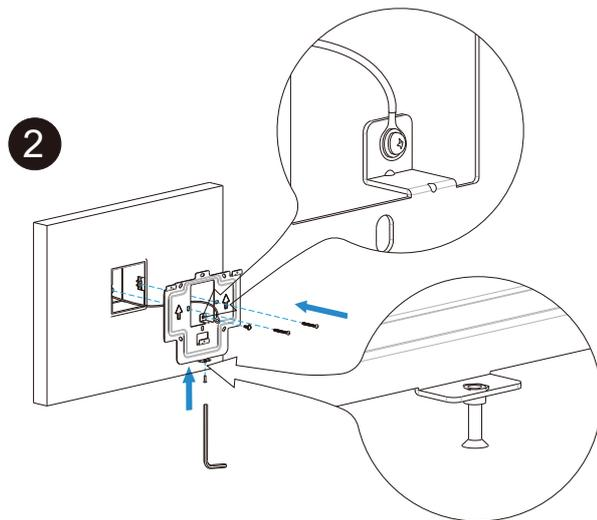
Twist M3x10.5 screw into the bottom hole of the wall bracket until the tail of which align to the edge. Then fix the wall bracket on the wall with two/four M4x30 screws. If there is a earth wire to be connected , use M3x6 screw to fix it on the wall bracket.
