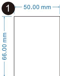
According to the position of the cable in the wall, dig out a square hole (height\*width\*depth = 66\*50\*50mm) that can accommodate all cables.
