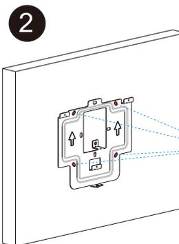
Align the square hole of the wall bracket with the hole dug out before, then mark the four fixation holes through bracket on the wall.
