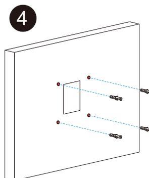
Once the fixation holes were made, insert screw fixing seats provided.
