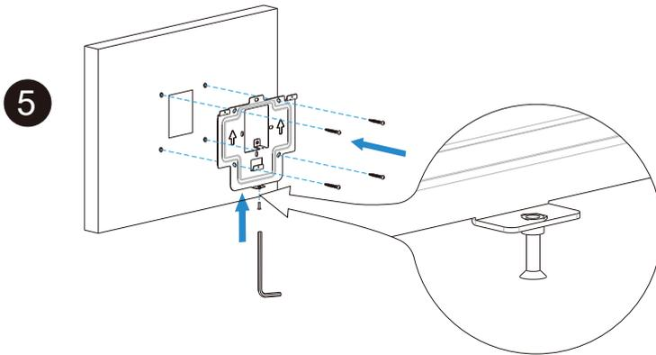
Twist M3x10.5 screw into the bottom hole of the bracket until the tail of which align to the edge. Then fix the wall bracket on the wall with four ST4x20 screws. If there is a earth wire to be connected, use M3x6 screw to fix it on the wall bracket.
