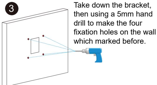
Take down the bracket, then using a 5mm hand drill to make the four fixation holes on the wall which marked before.
